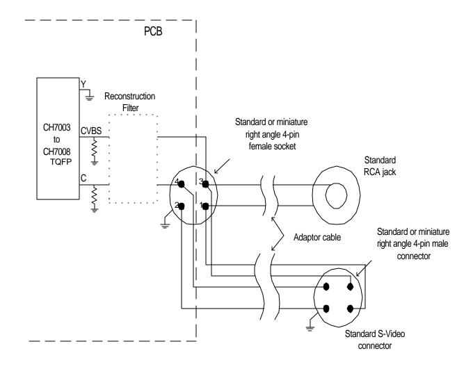
**Recommandation:** Please refer to Digi-Key or JAMECO for the standard socket & connector. Customer should be aware and consult the cable manufacturer regarding the EMI issue, when the small form factor custom made connectors & cables are required.
