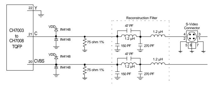
**Note:** All the VDD are connected to DAC power supply & GND are connected to DAC ground. Please refer to the data sheet for both VDD & GND pin's number. For PCB layout requirement, please refer to AN-24.
