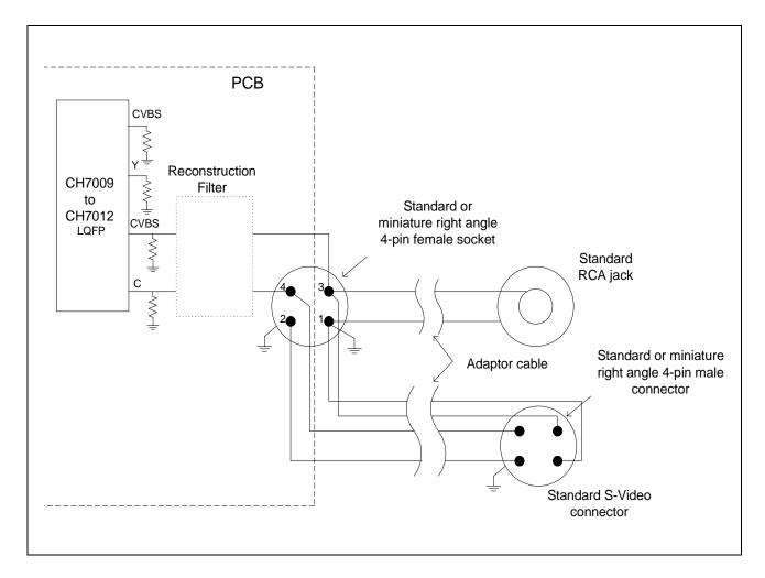
**Recommandation:** Please refer to Digi-Key or JAMECO for the standard socket & connector. Customer should be aware and consult the cable manufacturer regarding the EMI issue, when the small form factor custom made connectors & cables are required.
