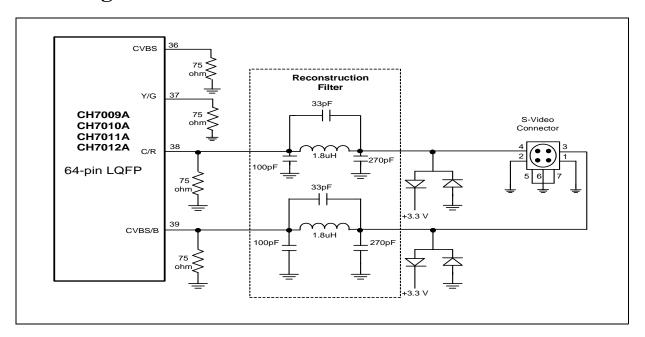
**Note:** All the VDD are connected to DAC power supply & GND are connected to DAC ground. Please refer to the data sheet for both VDD & GND pin's number. For PCB layout requirement, please refer to AN-34 (CH7009), AN-36 (CH7011), AN-44 (CH7010) and AN-45 (CH7012).
